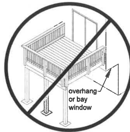
Figure 18. No Attachment to House Overhang with Ledger.
